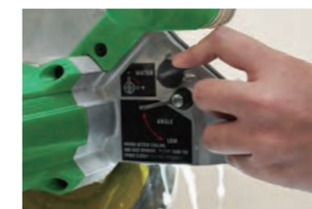
Water controls for volume / direction
